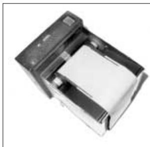
The film fed over the back to the take-up spool.
