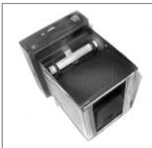
With the new spool in place and mask at film plane.
